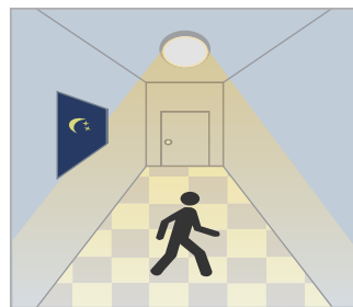
When motion detected, insufficient daylight, light ON.
